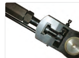
过载保护装置 Connection rod of overbear and anti-disconnection mechanism when overloading cutting it can protect cutting transmission system to prevent the machine
